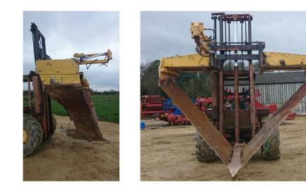
Prototype: JDN swamp excavator in combination with V-shaped plough
