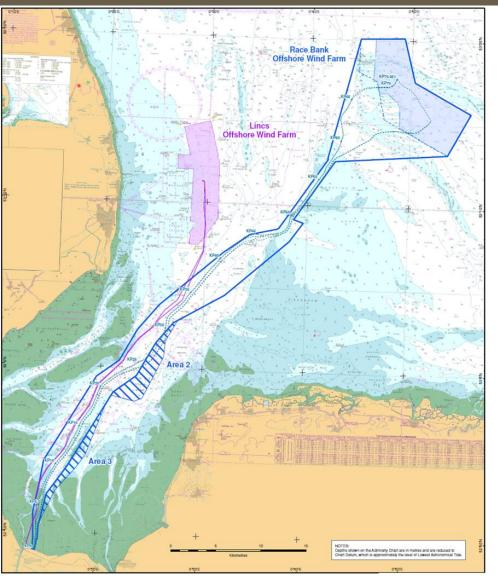
ROW01 project includes installation of approx. 2 x 71km 220kV submarine cable systems with integrated fibre optic cable between the offshore substation and the transition joint onshore and installation of a 6km long link cable.
